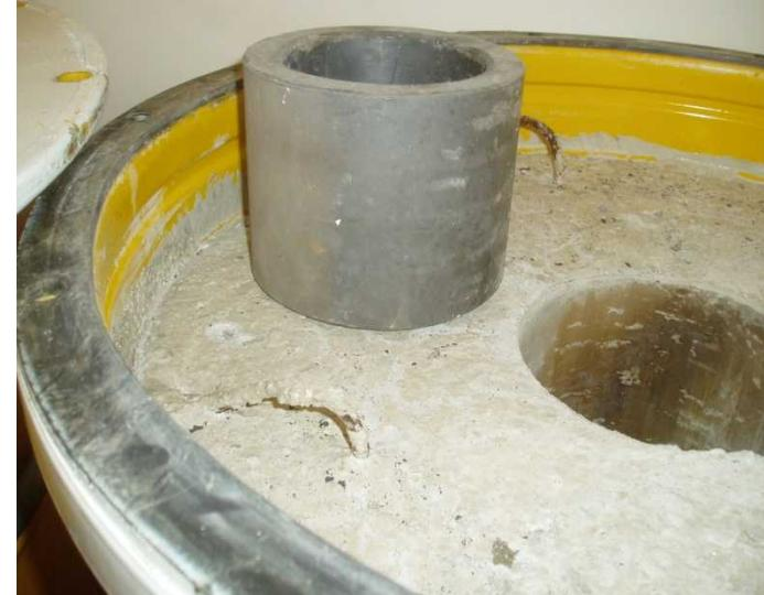
**Concrete lined drum with cavity for placement of sources/inner containers**
