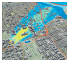
NISAC models different disaster scenarios such as a chemical/biological/radiological dispersion (left), damage downstream from a dam break (middle), and fallout from a small improvised nuclear device (right) in order to understand the effects and prepare responders to mitigate them.
