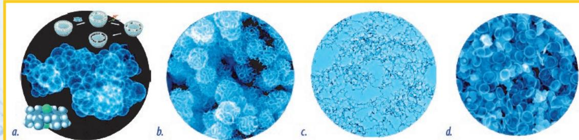
Some of the complex platinum nanostructures that can be produced, offering a wide range of potential applications in addition to hydrogen fuel cells; (a) platinum nanocage spheres template (b) nanospheres 'foam' composed of convoluted dendritic nanosheets template (c) 2 nm diameter nanowire networks template; and (d) platinum nanowheels template
