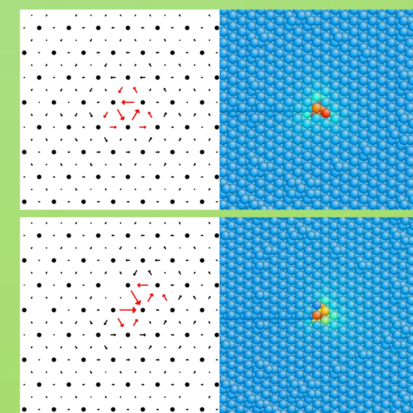
A possible interpretation of the split core structure is that the dislocation has divided into two partial dislocations that remain close together. This description explains how a fault forms for the large  $\chi$  angles.
