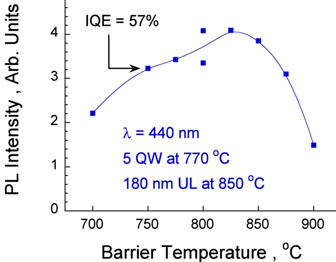
**Growth conditions** – 5 MQW structures grown on InGaN UL at 770 °C using different GaN barrier growth temperatures. Verified with XRD.
