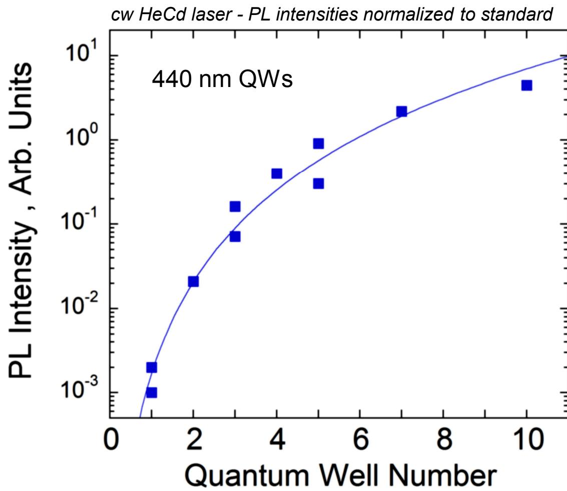
**Growth conditions** –  $n$  period InGaN MQWs at 770 °C, GaN barriers at 800 °C, pressure 300 torr. Structure verified using XRD.
