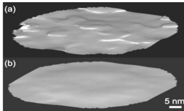
An isoconcentration surface based on atom probe tomography data illustrating the lower and upper interface of an InGaN QW.
