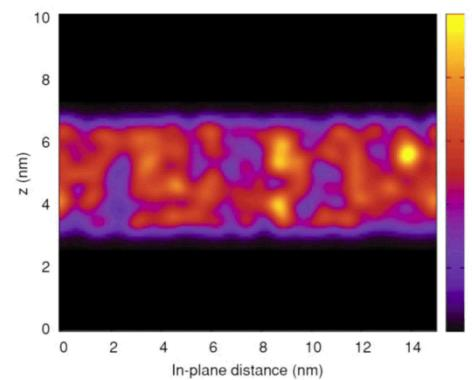
Indium fraction in a 3 nm thick QW with an average indium concentration of 25%.
