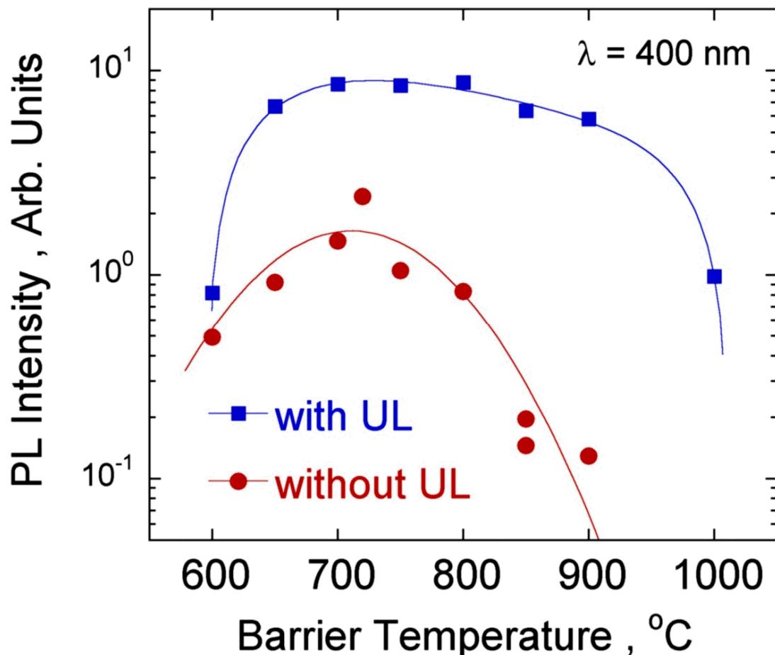
**Growth conditions** – 5 period MQWs at 790  $^{\circ}\text{C}$  with and without InGaN underlayer (UL), only GaN barrier growth temperature varied.
