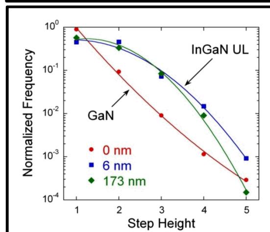
InGaN grown at 870 °C and has few V-defects
