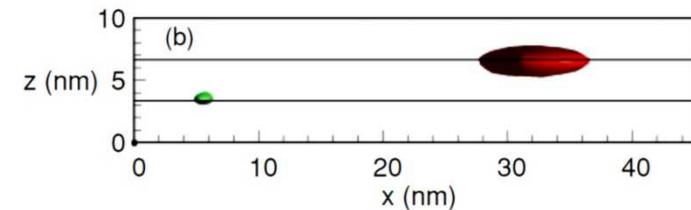
The calculated ground state probability density of an electron (red) and a hole (green).
