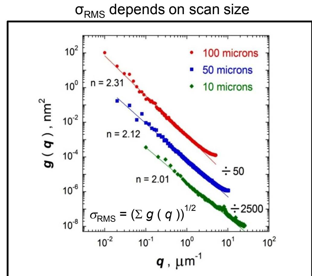
$n \sim 2$  - implies the smoothing mechanism is evaporation and recondensation of Ga atoms
