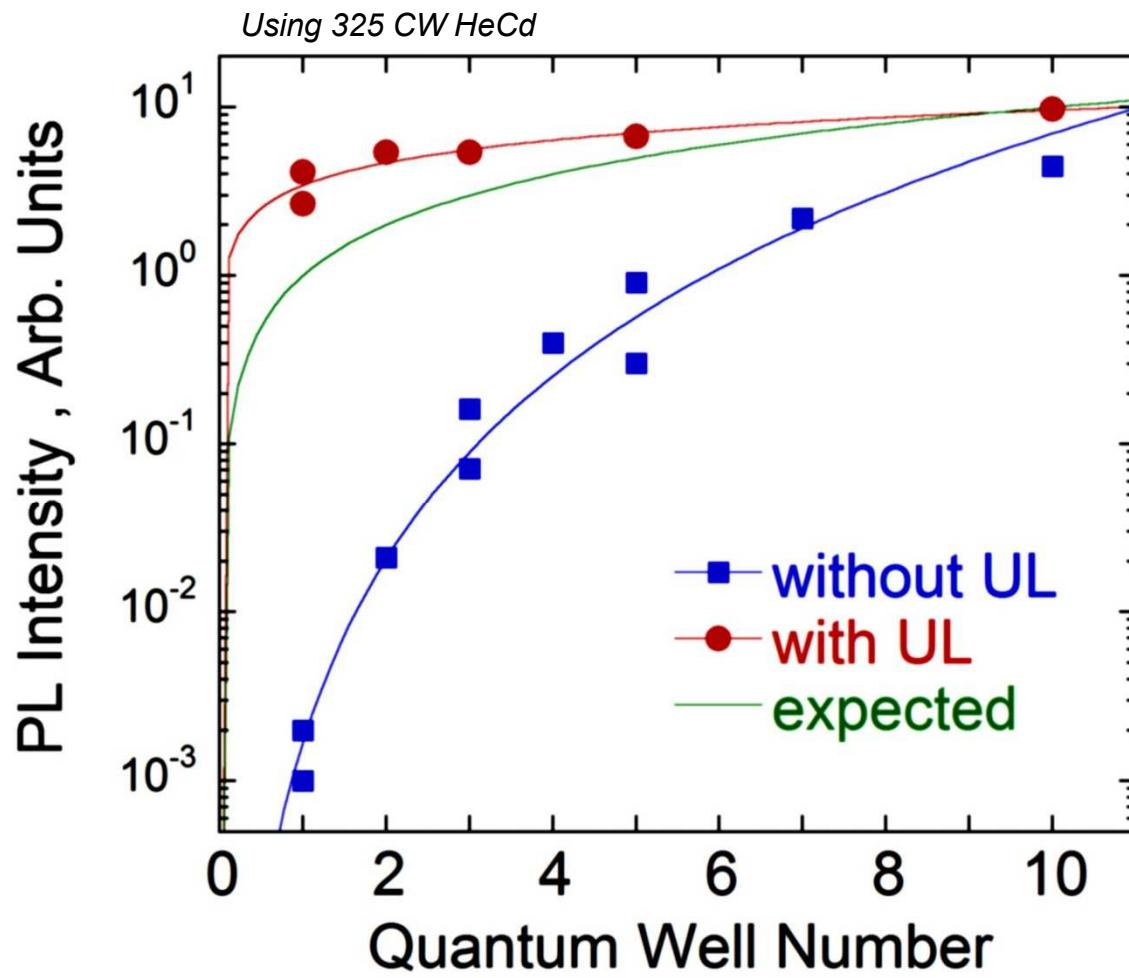
**Growth conditions** - InGaN underlayer (UL) at 850 °C, ~ 180 nm thick, 3 - 4% indium, pressure 300 torr. Verified with XRD.
