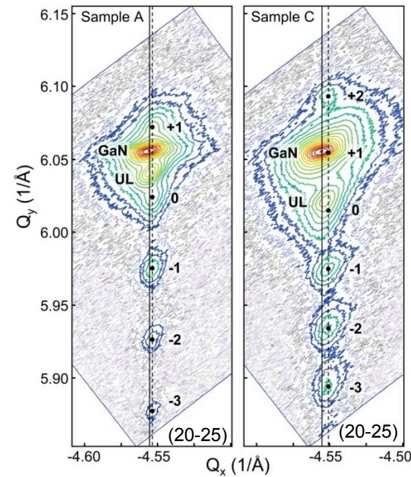
Sample A - InGaN UL and a 5-period  $\text{In}_{0.17}\text{Ga}_{0.83}\text{N}/\text{GaN}$  MQW – 2.8% per QW.
