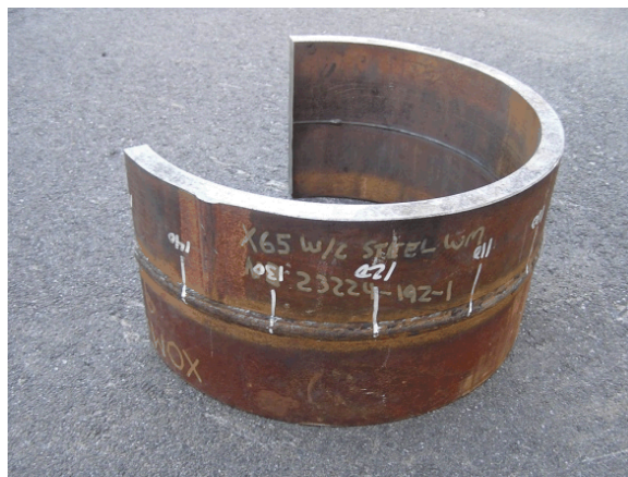
Figure 1. X65 steel girth weld supplied by industry partner.
