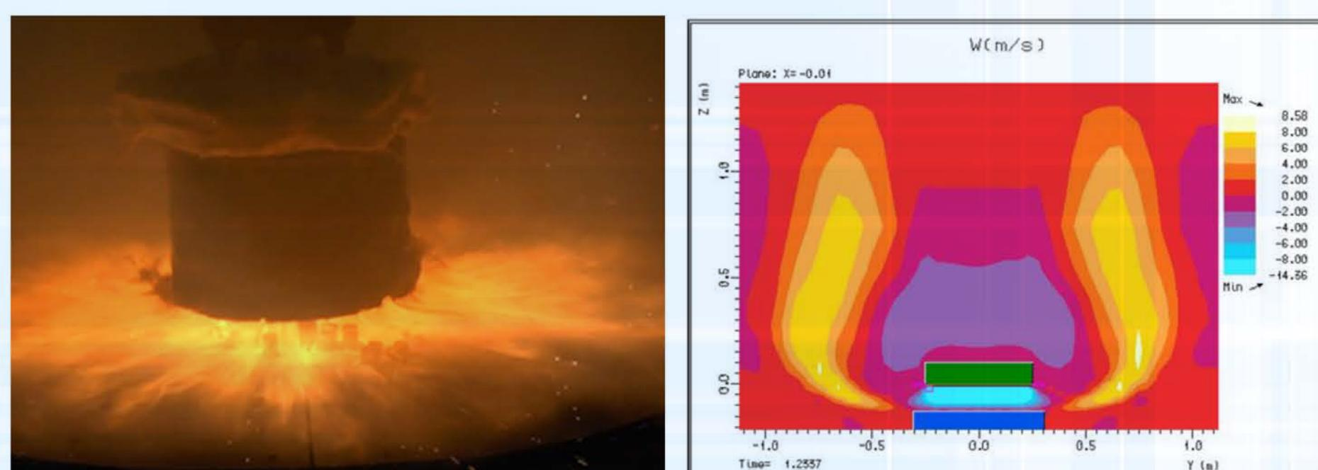
Burning in the small gap between a block of propellant and the ground underneath was previously modeled as a reacting flow between 2 parallel surfaces. However, real-time x-ray videos clearly show the development of burning cavities in the propellant created by the presence of small objects on the surface.
