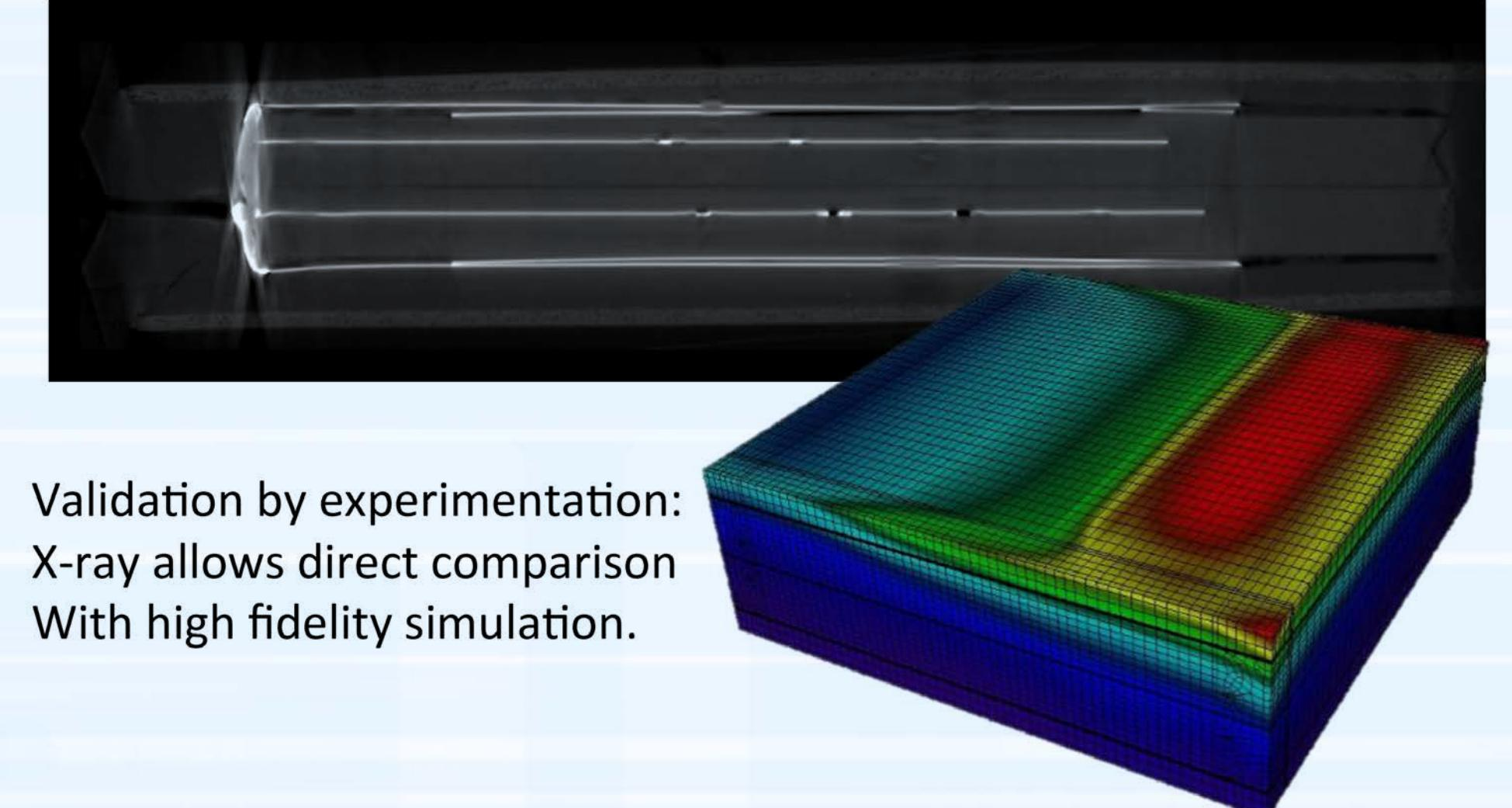
Often the final damage is destructive which doesn't allow a post-test analysis. The real-time attribute of the x-ray imaging systems allows a moment-to-moment evaluation
