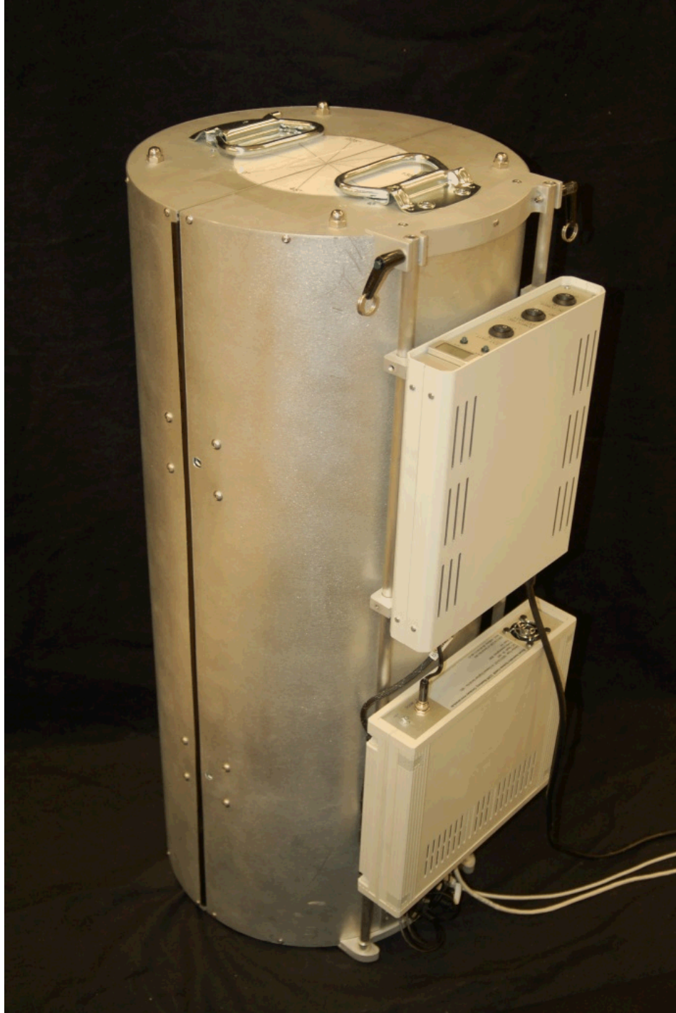
Figure 2. Power conditioning module (top) and sixteen-channel digitizer (bottom) mounted on the side of MINER. Power can be supplied from a wallplug outlet or a battery (110 W at 10-36 VDC). The only other component of the system is the laptop computer connected by the USB and Ethernet cables visible at the bottom-right of the photograph.
