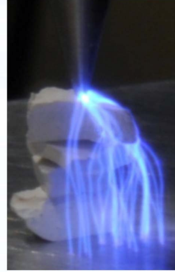
Recombination radiation from electrical breakdown with rutile in air a high dielectric material used in lightning arrester connectors (Zac Wallace & Jane Lehr)
