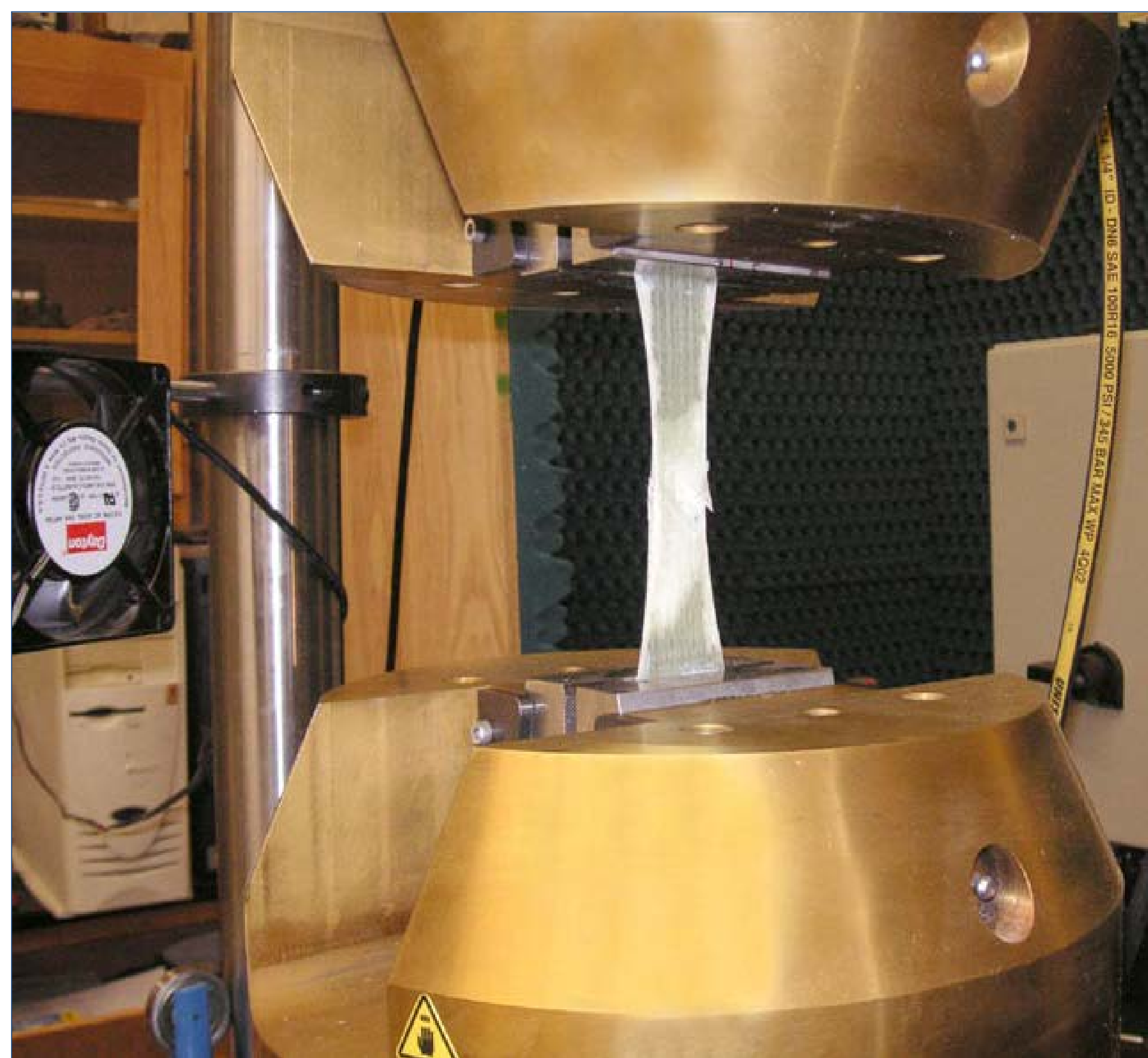
FIGURE 2- A COMPOSITE COUPON BEING SUBJECTED TO FATIGUE LOAD CYCLES IN ONE OF THE MONTANA STATE UNIVERSITY TENSILE TEST MACHINES
