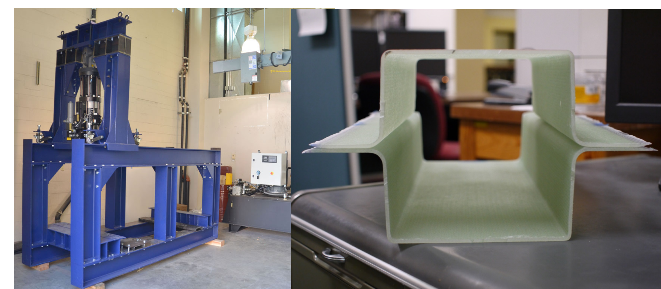
FIGURE 7 – THE SUBSTRUCTURE TEST FRAME (LEFT) WILL BE USED TO TEST NEW SUBSTRUCTURE TEST SPECIMENS (RIGHT) IN ORDER TO PROBE MATERIAL BEHAVIOR IN SHAPES AND LOADINGS THAT CANNOT BE DONE AT A COUPON SCALE.
