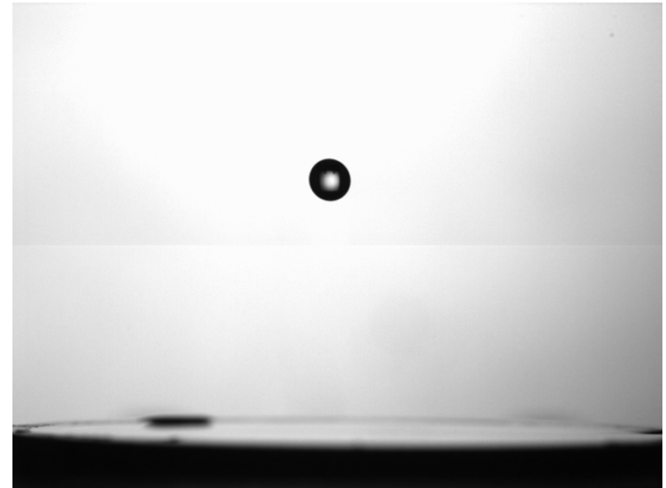
impact of a 3 mm water drop on a 2 mm water film (Guildenbecher et al, 2013, Exp. Fluids .)
