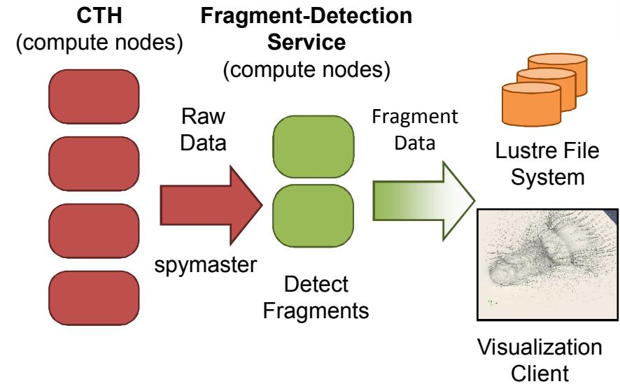
*Fragment detection service provides on-the-fly data analysis with no modifications to CTH.*
