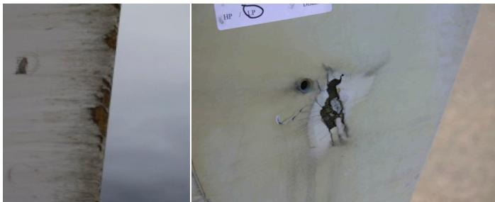
*Operational damage is also a cause of premature blade failure, whether it is from erosion of blade surfaces as shown on the left or lightning strikes as shown on the right.*
