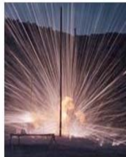
Figure 5-6. Photo of explosively-driven cylinder fragmentation and estimated average fragment size from three tests (Grady, 1982).
