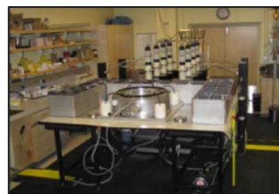
Figure 7-10. Photograph of the Veloce pulser used to produce magnetic ramp loading to peak pressures of about 200 kbars.
