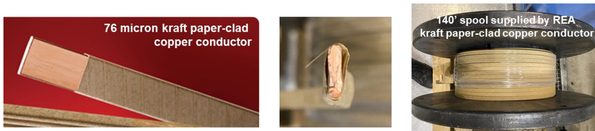
Figure 3-2. Images of Kraft paper spiral-wound, rectangular cross section, copper transformer conductors, of the type typically used for transformer windings shown in Figure 3-1.
