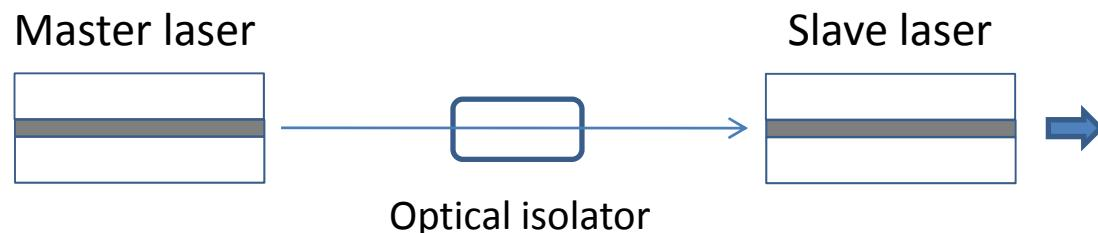
Removing the optical isolator simplifies experimental setups, but complicates theoretical analysis: coupled-laser system
