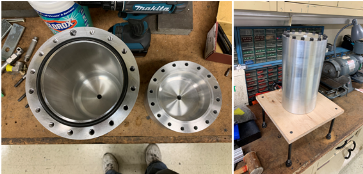
Figure 4: Thick-walled aluminum pressure vessel constructed for whole mask testing.
