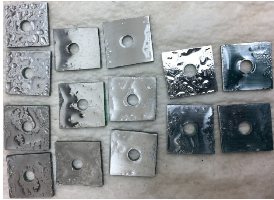
Figure 2: Picture of sprayed on disinfectant loading to a set of samples, \sim 0.25 \text{ L/m}^2 coverage.
