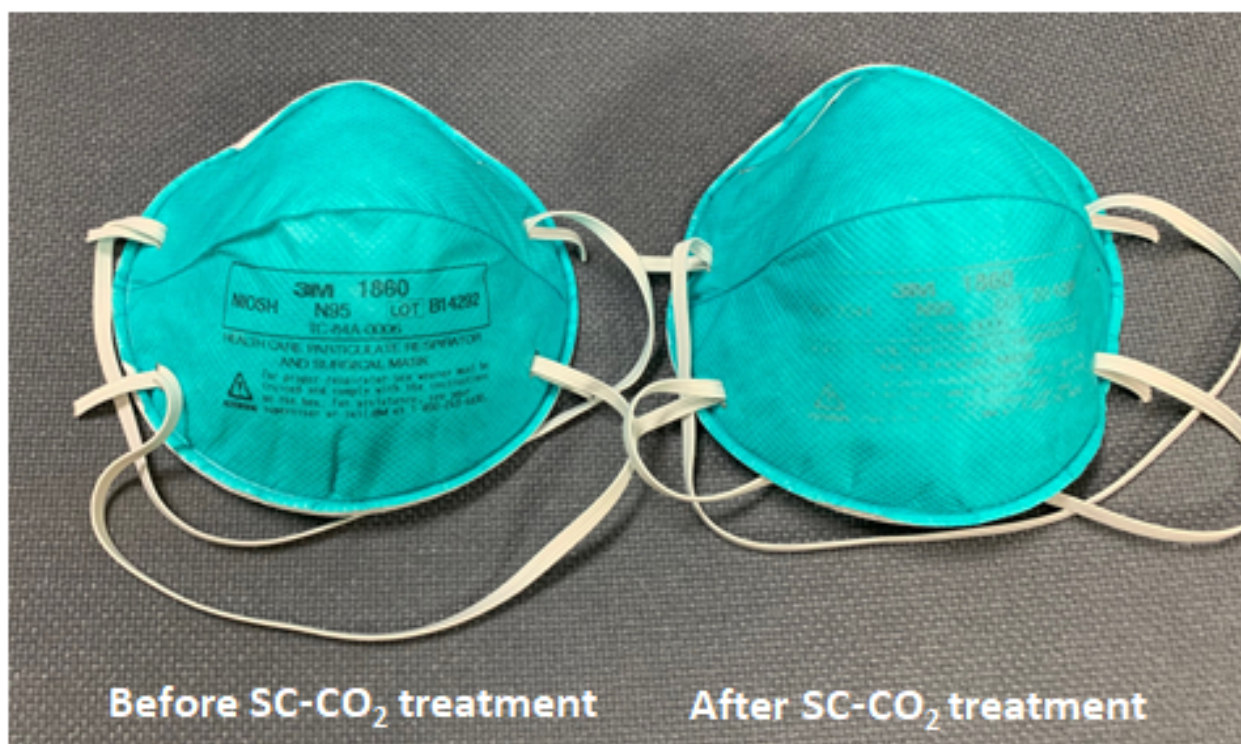
Figure 17: Before and after photos of a 3M type 1860 N95 mask subjected to one 60-minute supercritical CO 2 treatment cycle.
