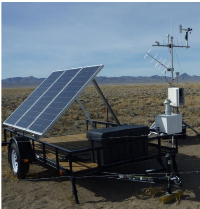
Figure A-4. Station 404, located along the north fence that bounds the Clean Slate II contamination area, includes a solar-powered air sampler and meteorological tower
