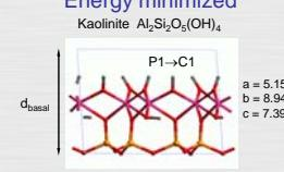
Geometry optimized structure of the unit cell of kaolinite based on CLAYFF; structure agrees with Bish (1993).
