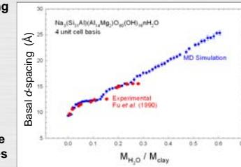
Swelling curve for the hydration of Na-montmorillonite derived from equilibrated molecular dynamics simulations (red) with experimental data (blue).
