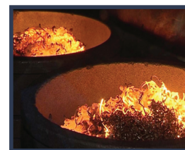
HEU metal is burned and converted into oxide
