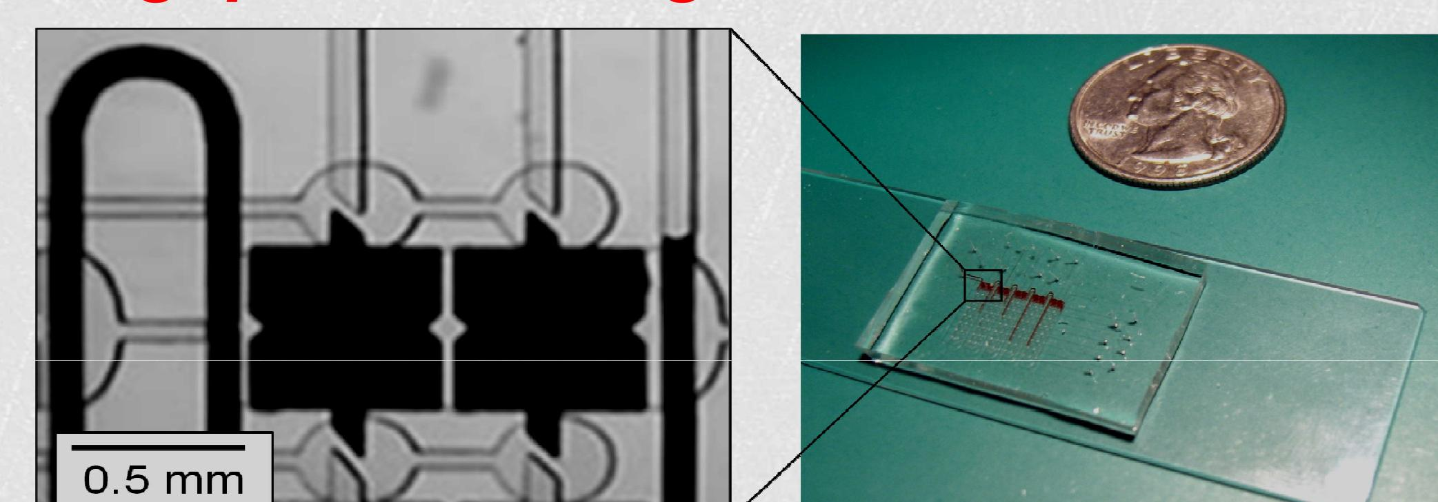
Microfluidic-based devices provide an optimal method to introduce RNAi libraries into primary cells within a portable and cost-effective platform. To this end, we are using microfluidic platforms that combine cell and siRNA array for the development of a high-level biocontainment compatible RNAi screening chip.
