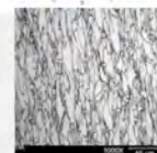
Point 13A is the harder spot with higher ASTM grain size, or small grain.
