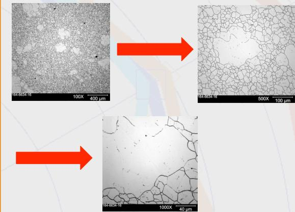
Bimodal grain structures were seen in the forging IAO164. A statistical representative ASTM grain size and hardness number is hard to reach because these large grains tend to be softer and have inconsistent ASTM grain size numbers in comparison to surrounding area.
