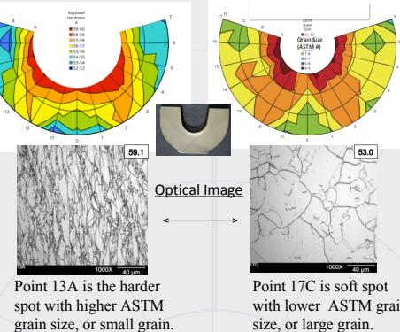
The grain size and hardness on the transverse cross section are related:
