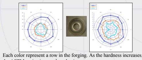
Grain Size is related to the degree of deformation:
