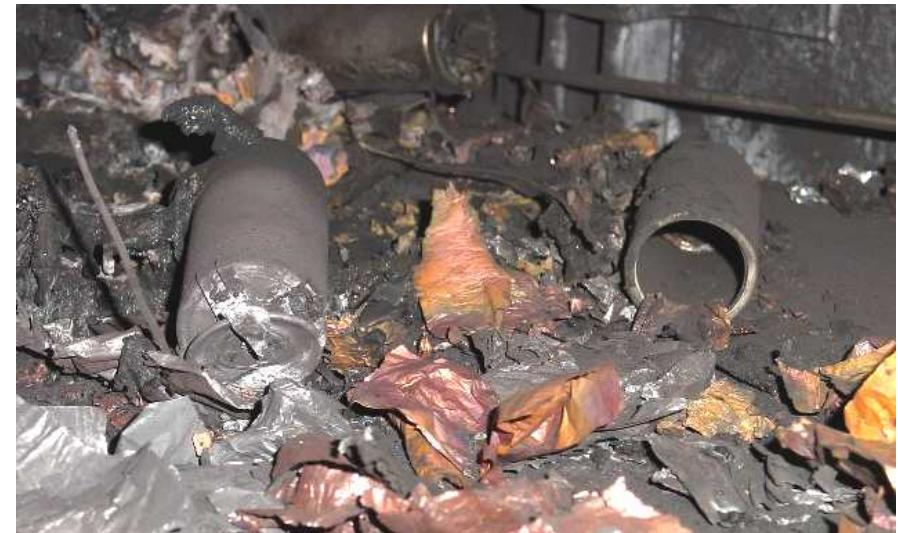
**Hazard Level 6 - Rupture**
