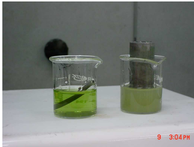
Corrosion of Hastelloy (left) and SARAMET (right) in 40% sulfuric acid at 90°C for 20 min.
