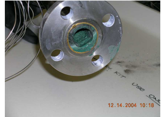
Hastelloy acid decomposer after 10 min. operation
