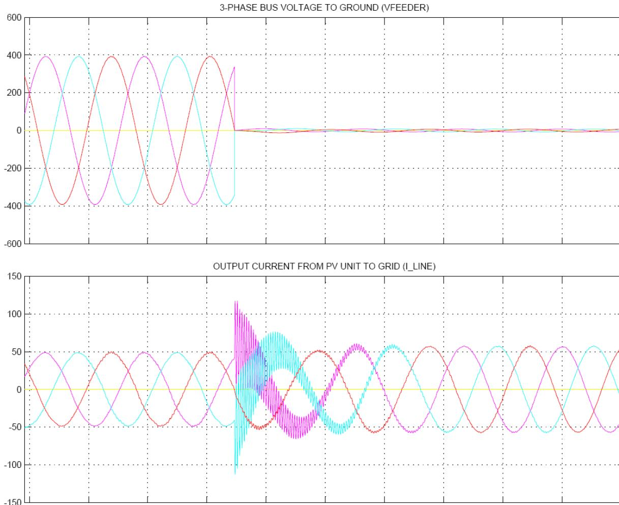
**Grid Voltage Monitoring Disabled to Allow Ride-Through During L-L-L-G Fault**
