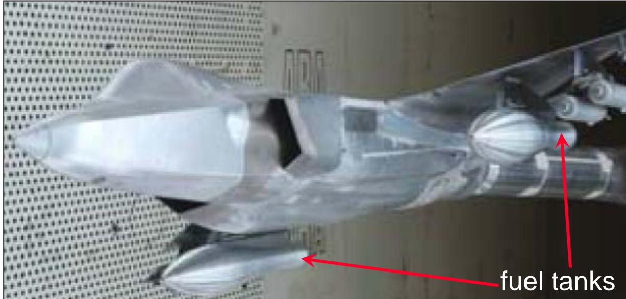
*This wind tunnel model of F-35 features an optimized external fuel tank.*
