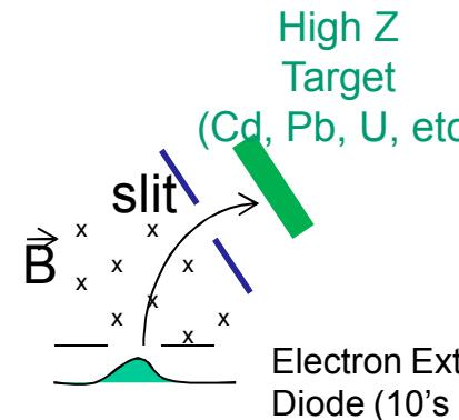
Low Voltage (100-300 keV, high current density ( $\text{kA}/\text{cm}^2$ ), pulsed electron diode in extractor geometry, magnetic field transport region, slit and 'thin' high Z target
