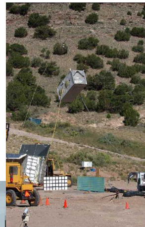
Full-scale drop test of TRUPACT III
