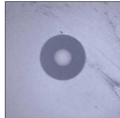
Fiber optic cable surrounded by cladding, magnified 400 times
