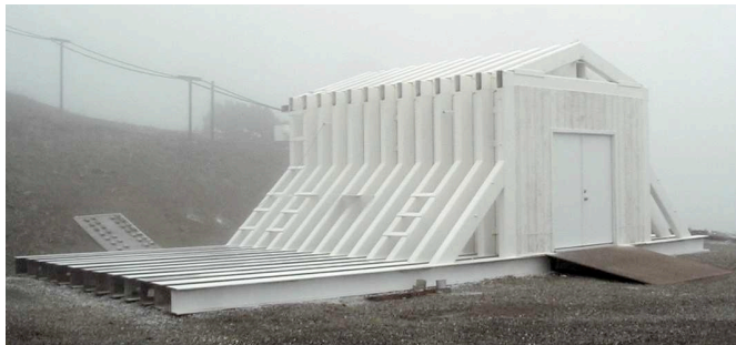
Maximum Overpressure Sub-Scale Warehouse - Open Wall on Front (2 sec ignition delay)
