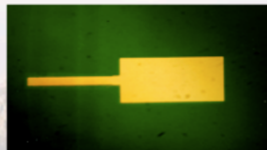
PZT-MEMs piezo cantilever beam for energy harvesting
