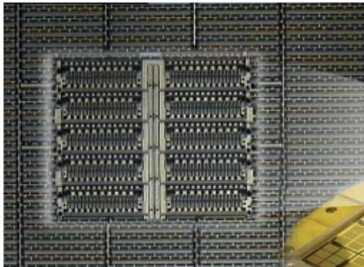
MEMS louvers manufactured at Sandia
