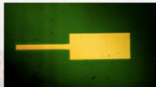
PZT-MEMs piezo cantilever beam for energy harvesting
