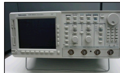
Tektronix TDS644A 500 MHz max analog bandwidth Up to 2 Gs/s 4 channels Up to 2000-sample record length per channel 8-bit digitizer
