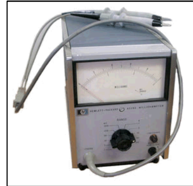
HP 4328 milliohmmeter Range: 1 mΩ – 100 Ω Accuracy: ± 2% of full scale Measuring frequency: 1000 Hz ± 100 Hz
