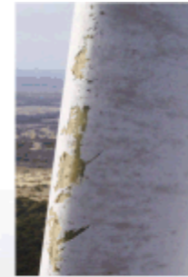
Leading edge blade erosion 4
