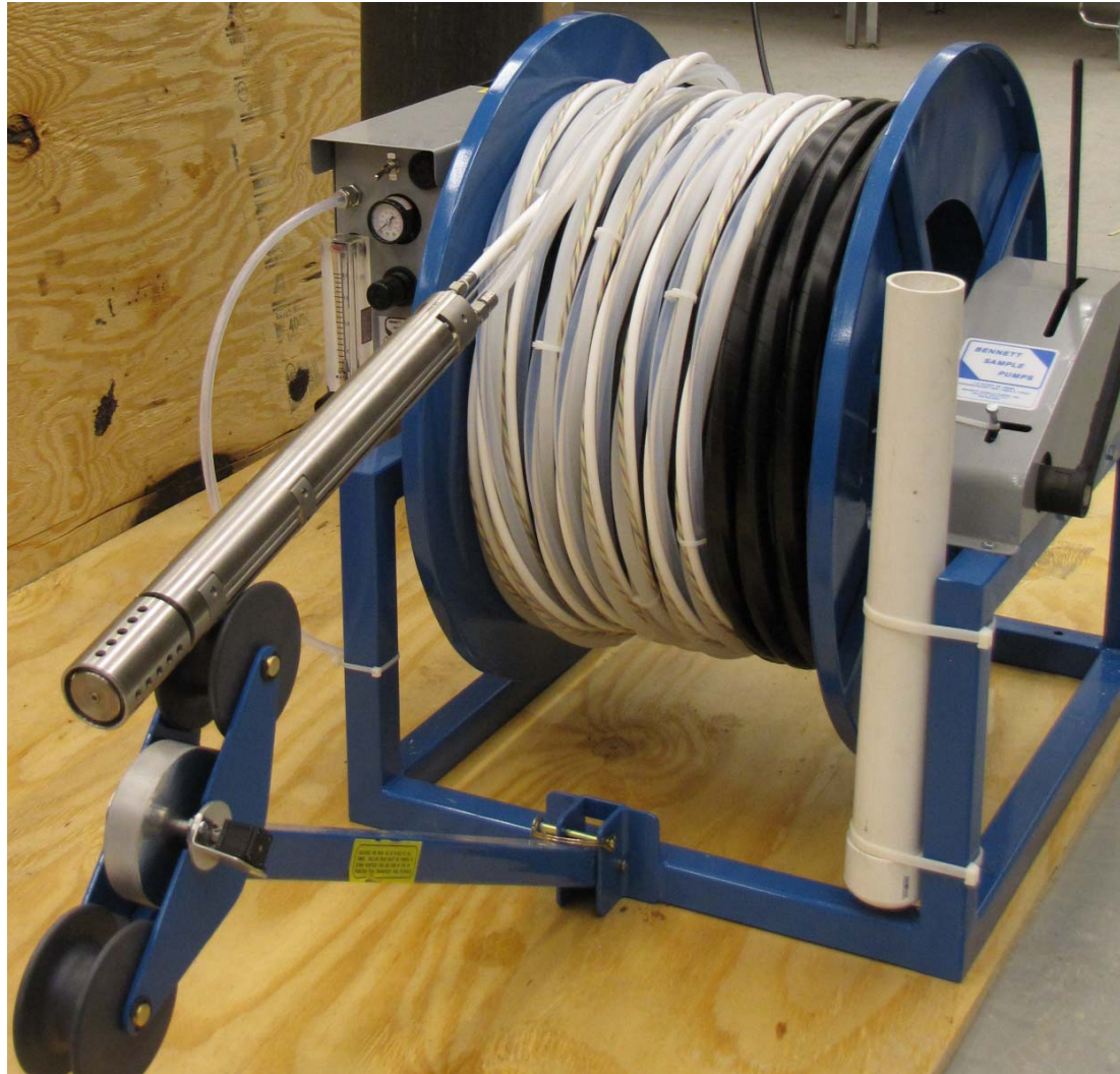
Pump, tubing and reel
