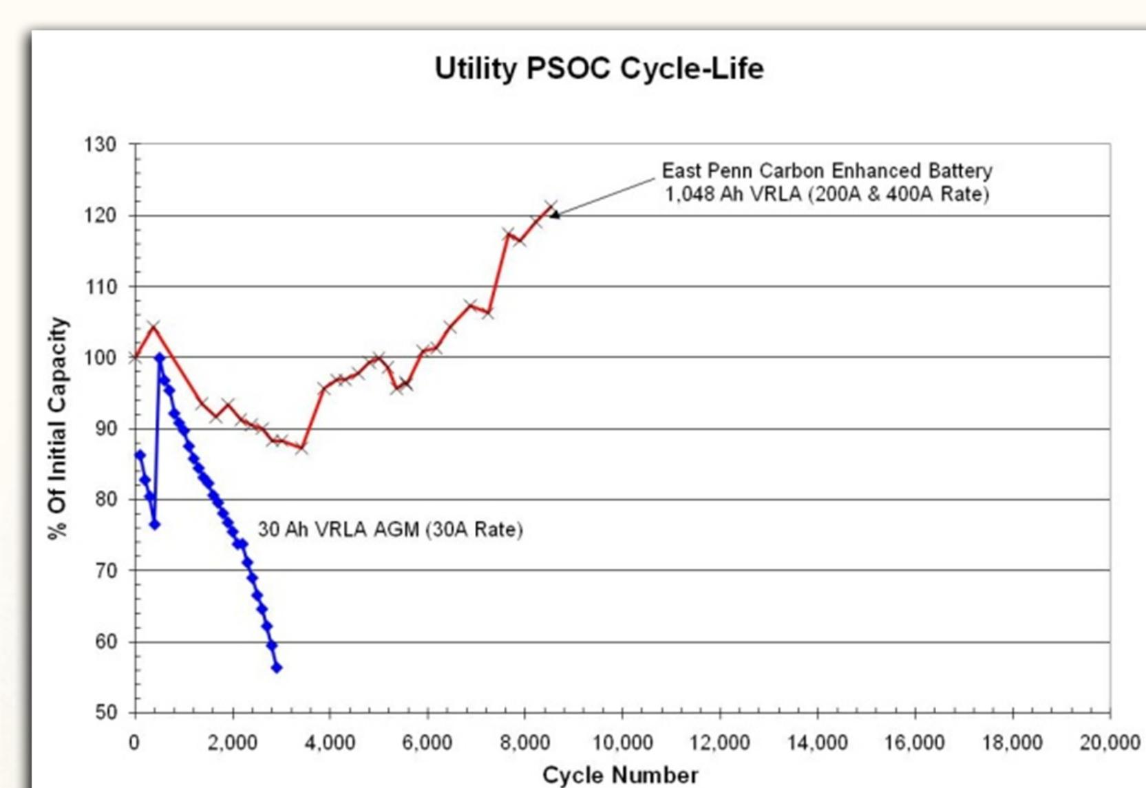
Carbon Enhanced battery capacity cycling at a partial state of charge.
