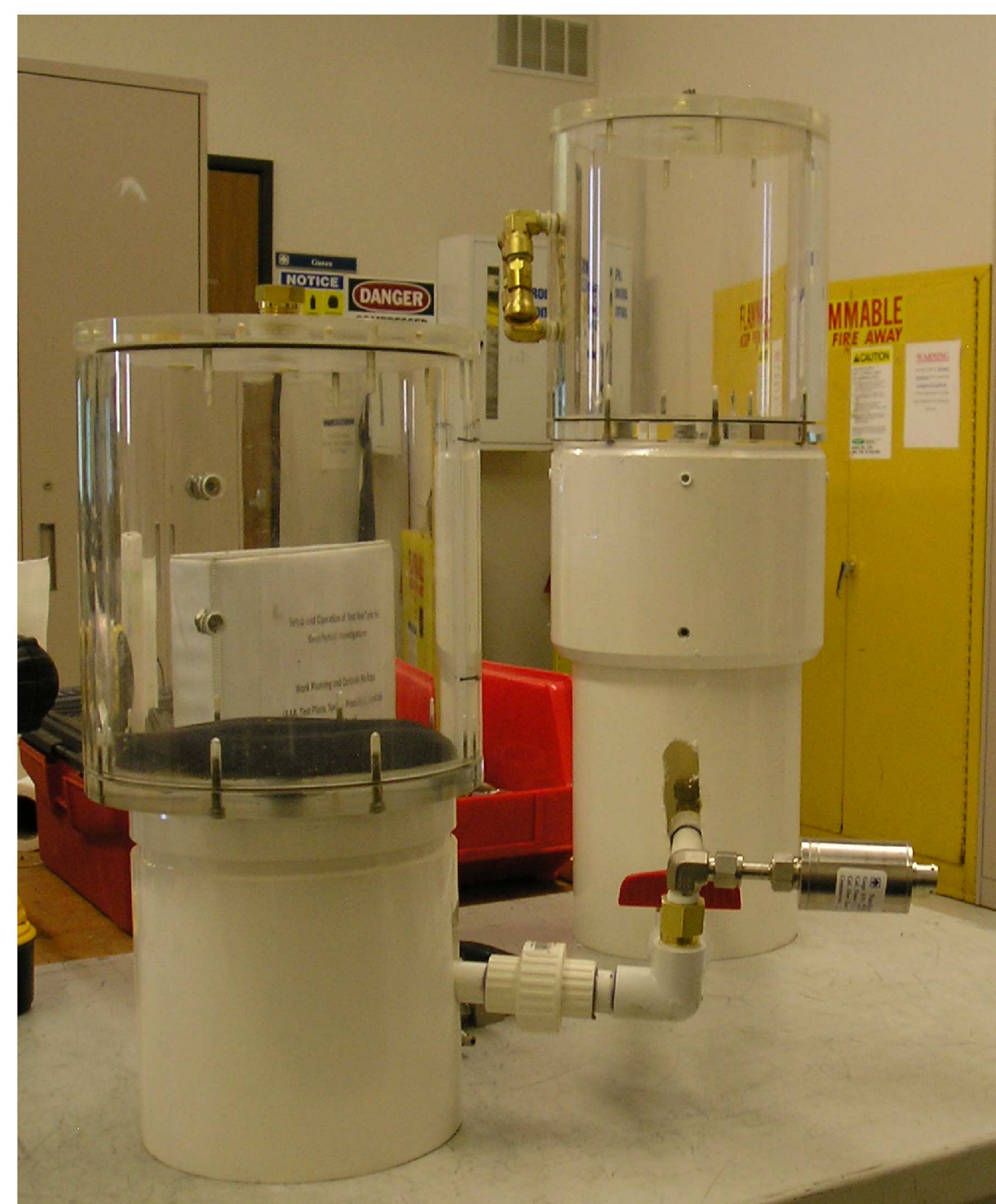
FIGURE 1: Permeameter showing sample holder, fluid reservoir, pressure transducer, and electrode ports.
