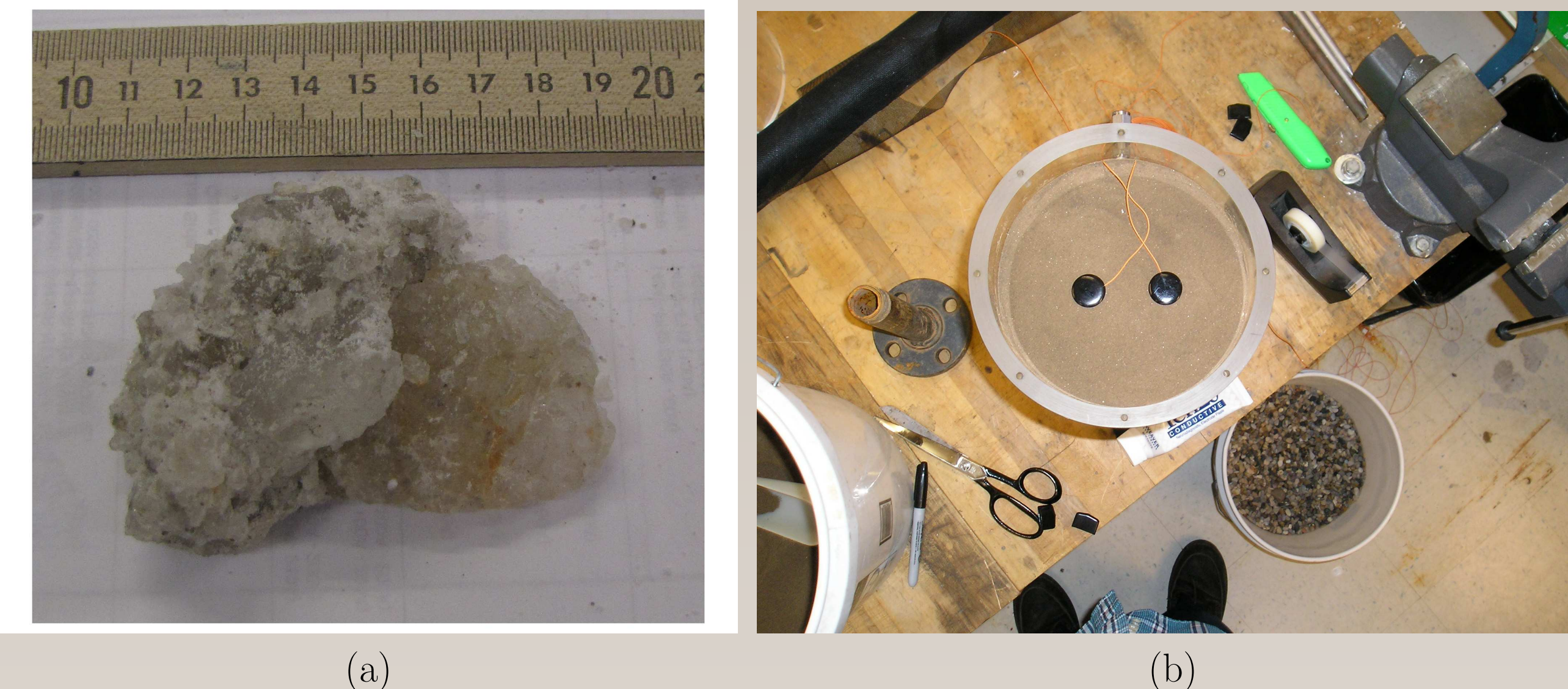
FIGURE 3: (a) Sample of crushed rock salt used in flow test. (b) Typical electrode placement on top of sample in permeameter.
