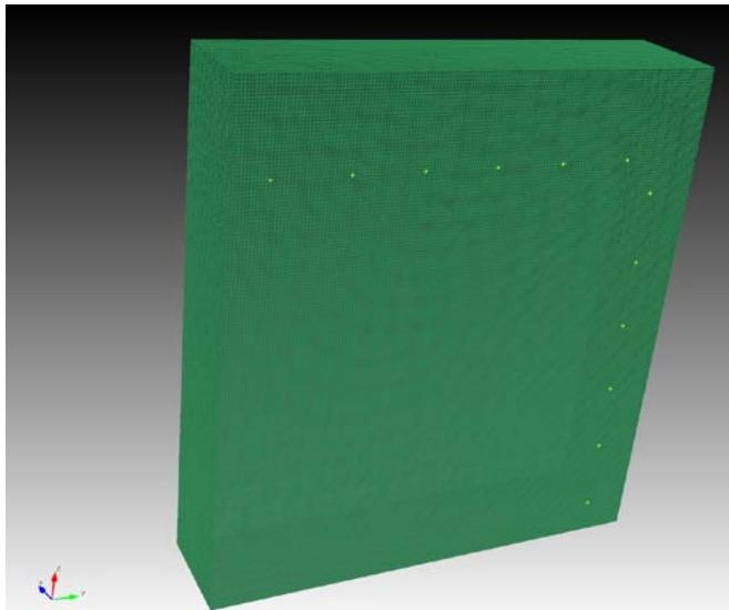
Meppen II-4 Model: no Z-displacement boundary condition constraint applied at light green dots. (Note:  $\frac{1}{4}$  model symmetry)
