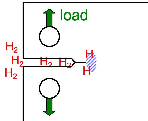
Rising-displacement fracture resistance is most conservative due to limited strain history
