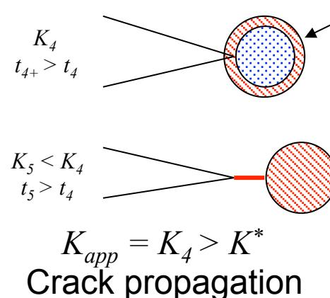
Large  $K_{app}$  is necessary to achieve crack initiation when load is applied in an inert environment
