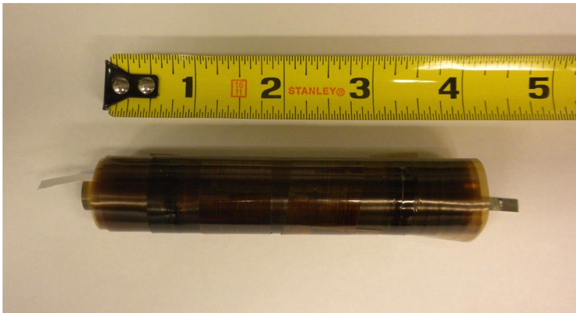
Figure 20. 3 ft capacitor (post rolling) of extruded 10% (w/w) trioctyl trimellitate in S-POW.
