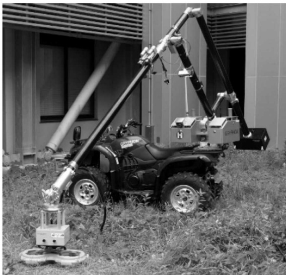
Figure 4: Mobile robotic ATV-mounted NQR detection system. Adapted from Ref 15.
