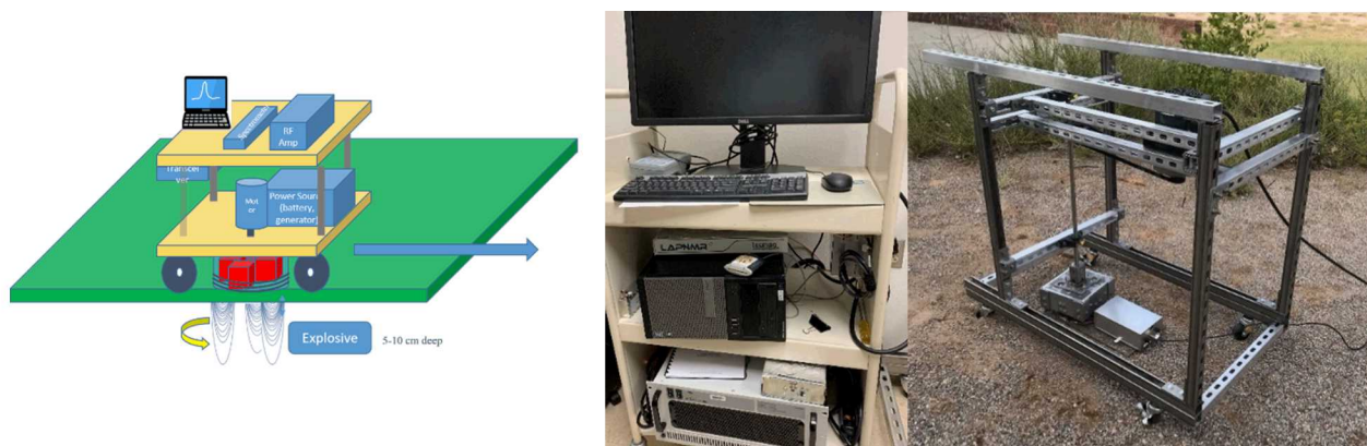
Figure 22: Left: Consolidated electronics and rotating magnet stage concept. Right: electronics cart and rotating magnet stage prototype in the field.
