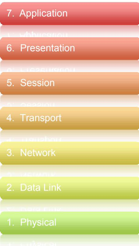
The diagram illustrates the OSI 7 layer model as a vertical stack of seven colored layers, each with a corresponding number and layer name. The layers are: 1. Physical (green), 2. Data Link (light green), 3. Network (yellow), 4. Transport (orange), 5. Session (dark orange), 6. Presentation (red), and 7. Application (dark red). Each layer is partially reflected below it, creating a shadow effect.
