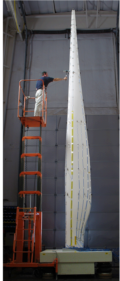
A test is performed at Sandia to validate a structural model of the Sandia Blade System Design Study (BSDS) blade concept. The innovative flatback airfoil technology demonstrated in the Sandia BSDS program has been adopted in industry by several blade manufacturers. Todd Griffith was the lead for the modal test effort shown in the photo.
