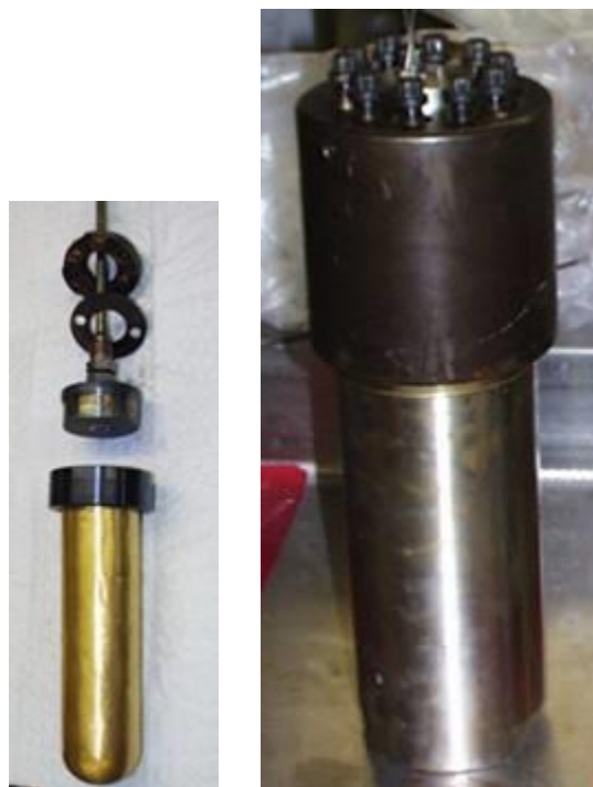
Figure 3-1. Gold bag (left) and gasket confined closure reactor (right) – Courtesy, Florie Caporuscio, Los Alamos National Laboratory.
