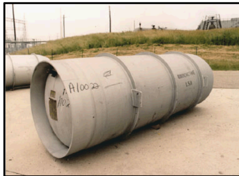
UF_6 is transported in special 12 MT, 48" dia. steel cylinders like the one shown in this Department of Energy photo.
