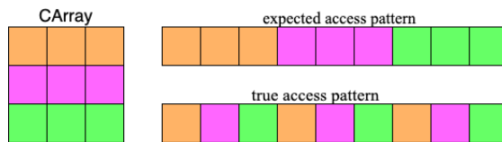
Figure 4.29. The figure shows a 2D CArray . As explained in section 3, the memory layout for a CArray is contiguous in memory row-wise. In order to maximize cache usage, the access pattern should be row by row. However, for a matrix-matrix multiply operation, the right matrix traverses the columns. Elements already loaded into cache are ignored and more memory loads are needed per calculation. The bottom array shows the actual access pattern for the latter matrix.
