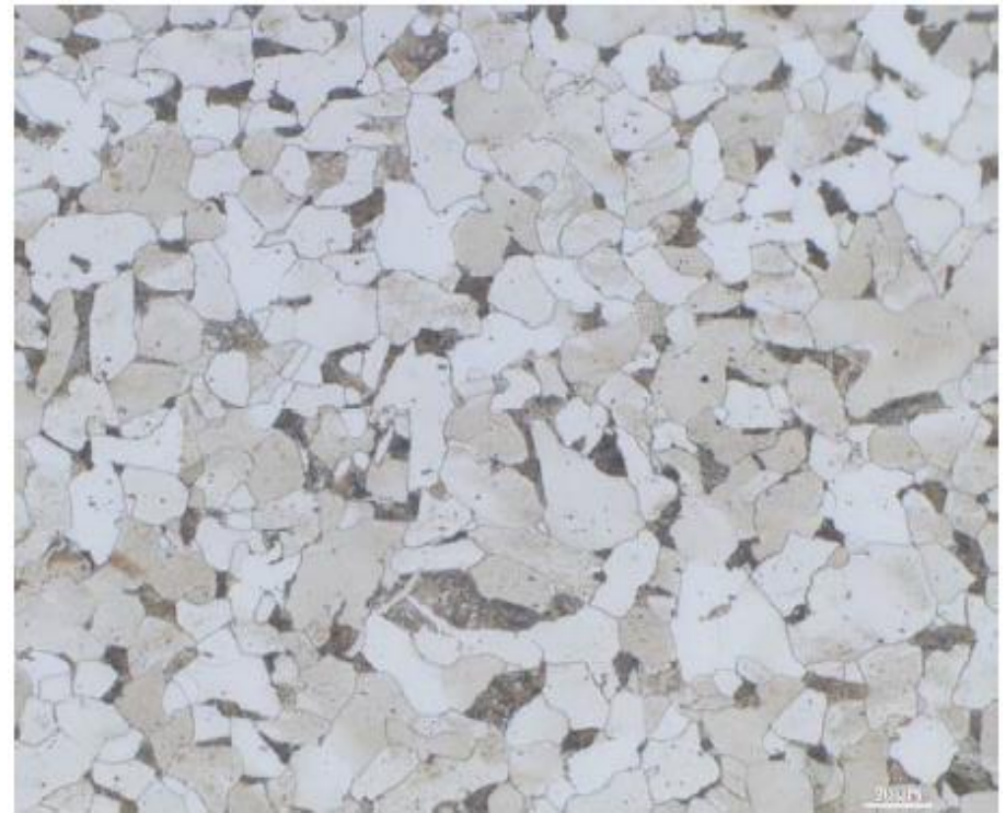
Figure 2. Optical microscope images of polished and etched cross section of the lid of the second Li pre-heater.
