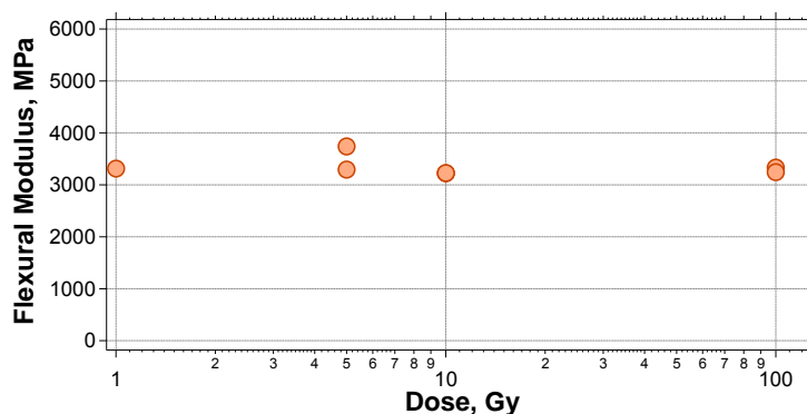
Fig. 19. Three-point-bend data for the flexural modulus of Torlon® 4203 irradiated to varying doses.
