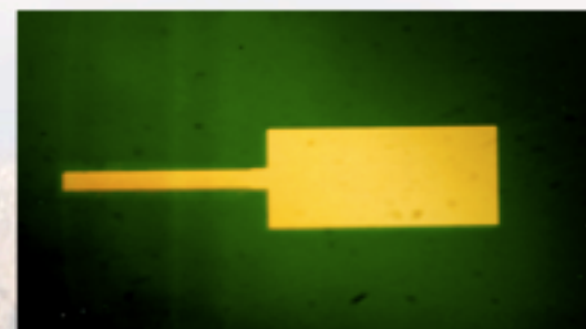
PZT-MEMs piezo cantilever beam for energy harvesting
